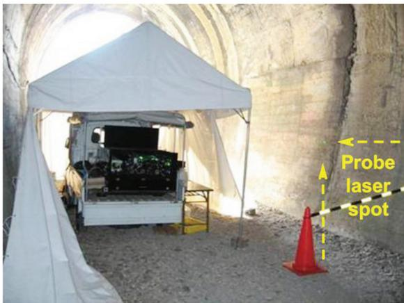
Fig. 6 The first tests in real tunnel. Inspection distance—2.5 m.
