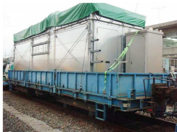
Fig. 22 The system with the sound-proof cover.
