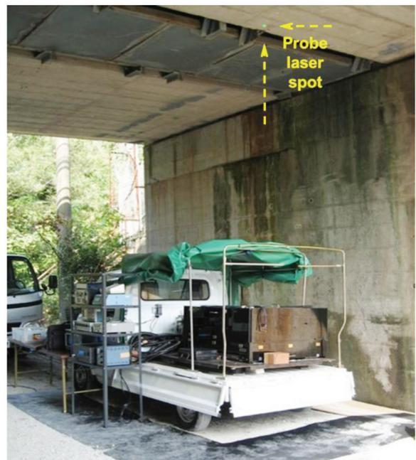
Fig. 17 The system is under Shin-kansen line bridge.
