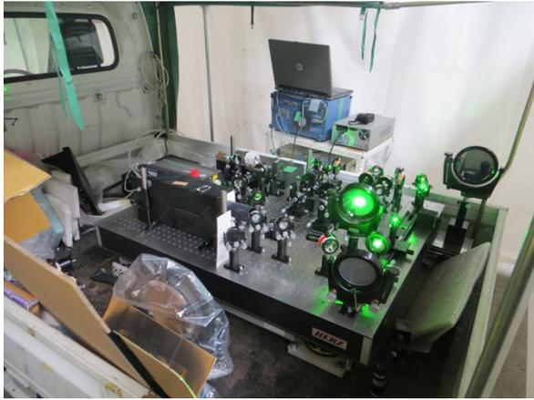
Fig. 5 Two-beam probing system under highway bridge.
