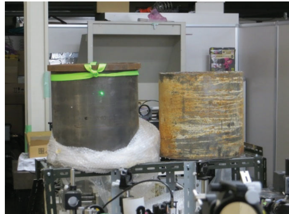
Fig. 1. Original pipe samples used in the tests. The “unused” sample has rims on its ends.
