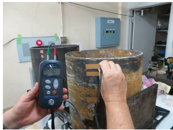
Fig. 5. Pipe wall thickness measurement with the use of contact ultrasonic gauge.
