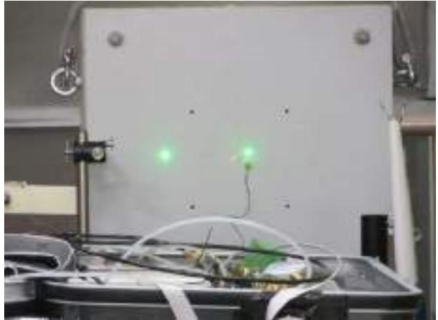
Fig. 11. Laboratory sample under inspection. Two green points are probe beams. Small red point is impact beam position. Four black points are corners of inner defect.
