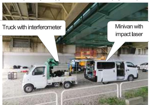
Fig.18. Two-carrier mobile system prototype.
