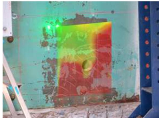
Fig.24. The defect area and its 2-D map.
