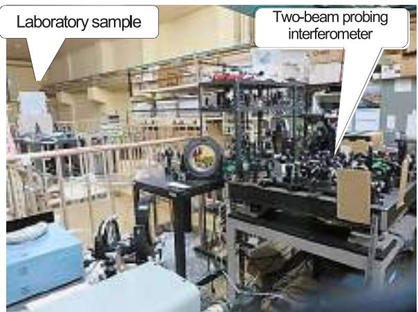
Fig. 9. Laboratory setup. Interferometer and concrete sample.
