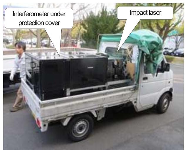
Fig.19. One-carrier mobile system prototype.
