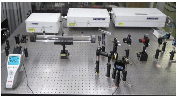
Fig. 3. Experimental setup of the SBS pulse compression system.
